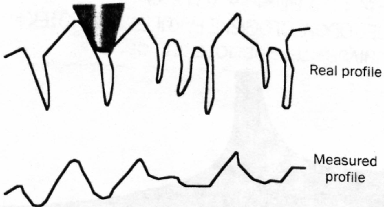
**Fig 1** Diagram of the influence of tip radius on the measured profile. A radius that is too large will result in a loss of information.
