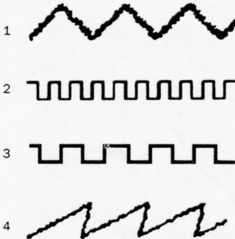
**Fig 6** Four different profiles with the same average height deviation ( $R_a$ ).
